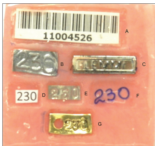
Figure 2: Inclusion labels: (A) Barcode Sticker (B): Lead Foil (C): Ni-Cr Plate (D): Paper (E): SS band (F): OHP Sheet (G): Brass palette
