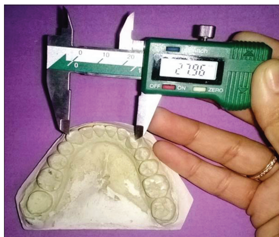
Figure 4: Photograph showing intercanine measurement on a cast
