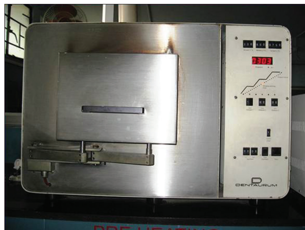
Figure 1: Electric furnace used to subject the teeth to desired temperatures
