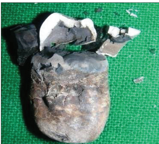
Figure 5: Zinc oxide eugenol at 600: macroscopically dark gray with cracks and dimensional contraction by loss of water, agglomerated particles of zinc
