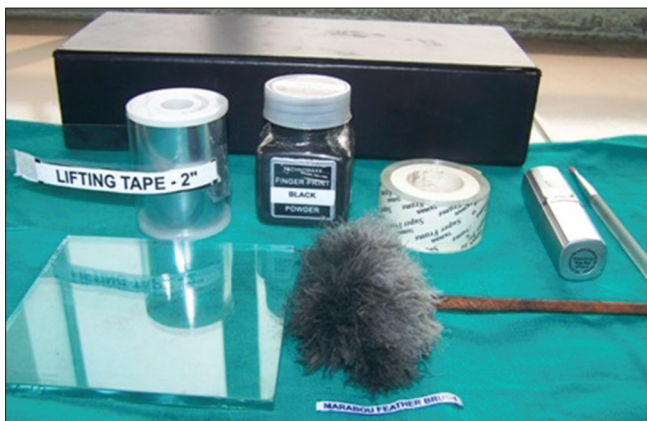
Figure 1: Materials used for development of latent and lipstick print: Black fingerprint powder, marabou brush, lifting tape 2" wide lifting take, glass slab, standard company lipstick, lipstick brush, cellophane tape
