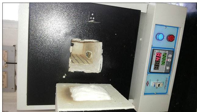
Figure 2: Teeth were held in a crucible and heated in a temperature controlled electric furnace
